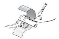
Install the temperature sensors with cable ties with the heat conducting paste and aluminium tape. Then insulate with supplied insulation tape.
